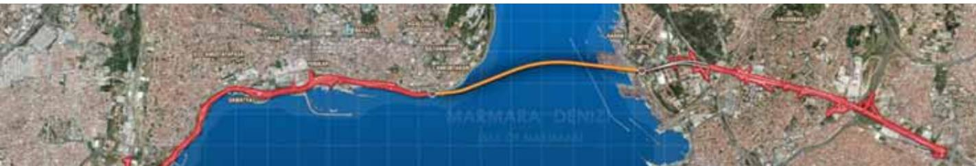
The Eurasia Tunnel Project is a 5.4-km twin-deck bored motorway tunnel that will cross the Bosphorus at its southern end running from Sultanahmet on the European side to Selimiye on the Asian side of Istanbul.
